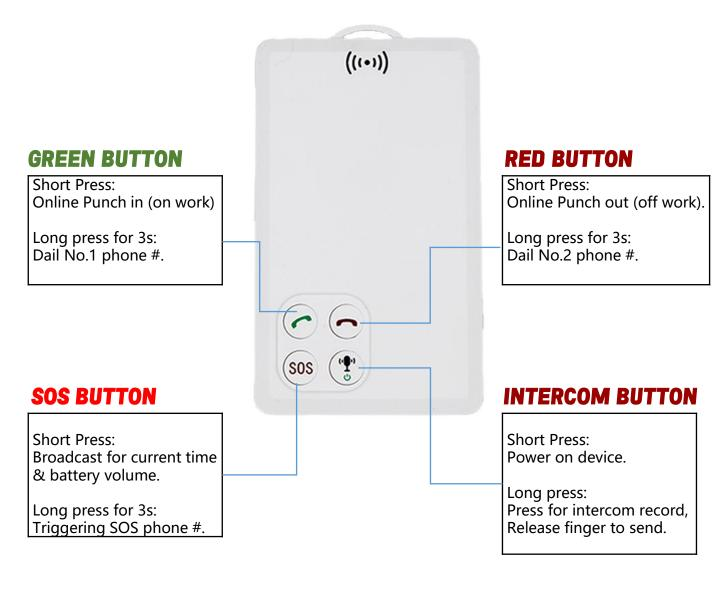
POWER OFF: Long press Green Button + Intercom Button POWER ON automatically when charging device
